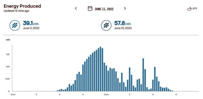
One week earlier on June 11, 2022 it was a mostly sunny morning turning to overcast for the afternoon with a couple of sunny breaks. The day generated 39.1 kWh) over the maximum period of the day (5:30 am to 8:30 pm) but still exceeded my yearly-averaged 36 kWh consumed per day.
