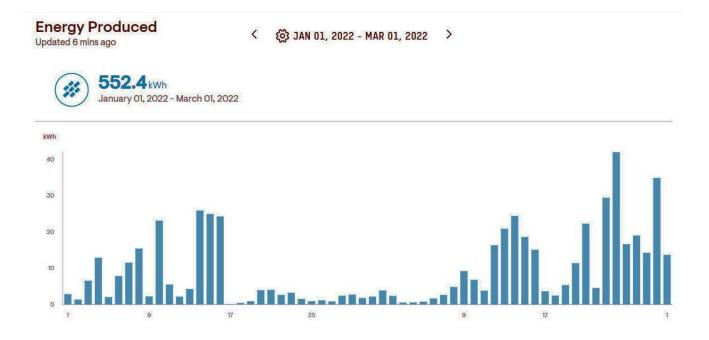
The system generates power throughout the winter but obviously much less than during summer time. On Jan. 17, 2022 there was zero-kWh generated when we had the massive snowfall in less than five hours. It took three days before the system started to deliver power again since most of the panels were covered in snow and ice. It took more than three weeks for the panels to start generating meaningful power with a peak on Feb. 24/22
